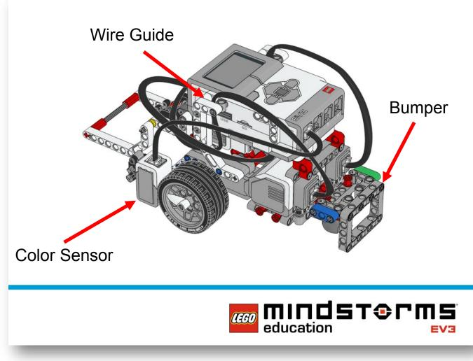
After you have verified your robot has a medium motor and end effector installed, you may begin Task 1 of Lesson 7. Task 1 directs you to modify the robot with the addition of a color sensor (for line following), some wire guides and a bumper. The building instruction to do this are found <u>here</u>.
